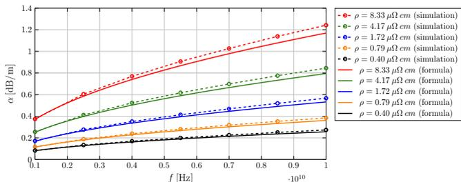
Fig. 9. Ohmic attenuation for different  $\rho$  - Pucel [5] formula in comparison to simulation results
