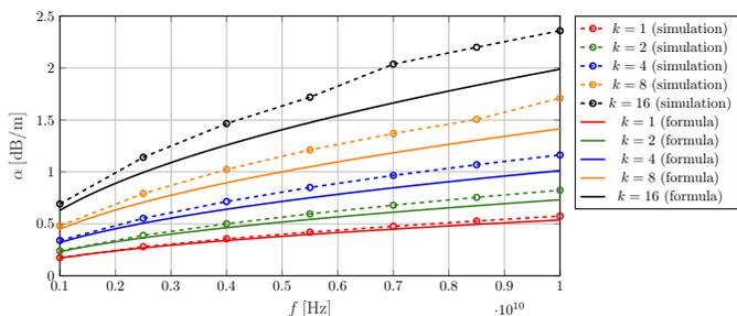
Fig. 8. Ohmic attenuation for different  $k$  - Pucel [5] formula in comparison to simulation results
