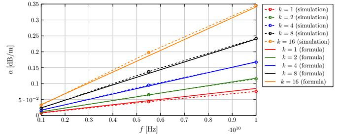
Fig. 6. Dielectric attenuation for different  $k$  - Schneider [6] formula in comparison to simulation results
