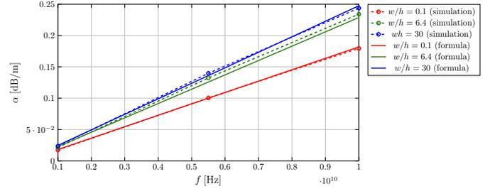
Fig. 7. Dielectric attenuation for different  $w/h$  - Schneider [6] formula in comparison to simulation results
