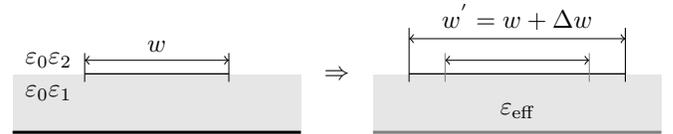
Fig. 2. Transformation of the geometry and applying an effective dielectric constant to calculate line impedance  $Z_0$ . Note the assumption  $t = 0$  to calculate line impedance.
