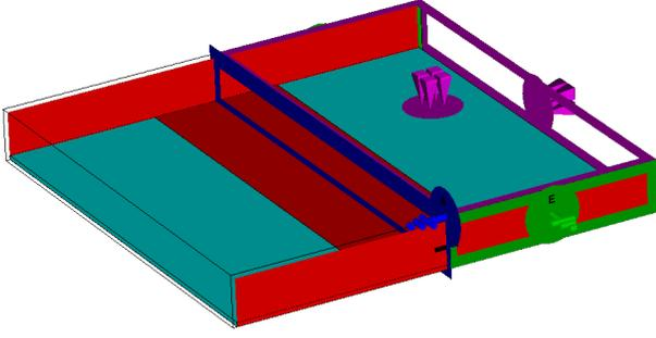
Fig. 4. CST MICROWAVE STUDIO® [1] - simulation assembly and boundary conditions. Colors: green - electrical boundary, purple - open boundary, blue - magnetic symmetry plane
