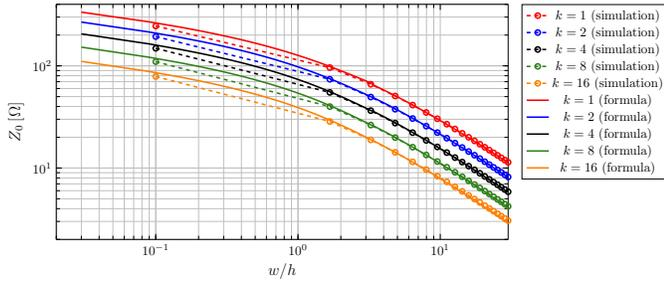
Fig. 5. Line impedance for different  $k$  - Heinrich [3] formula in comparison to simulation results
