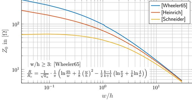
Fig. 3. Comparison of line impedance calculation by various authors
