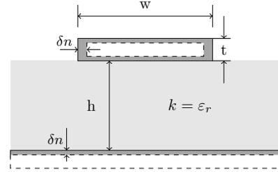
Fig. 1. Illustration of the example geometry with specified parameters according to the listed notation.
