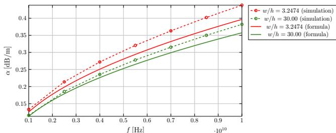
Fig. 10. Ohmic attenuation for different  $w/h$  - Pucel [5] formula in comparison to simulation results
